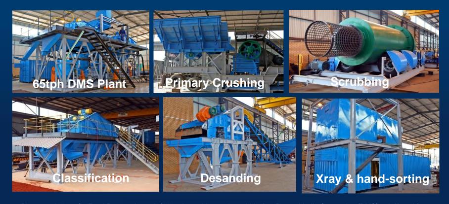
Plant consisting of a Feed Preparation unit (200 tph crushing and scrubbing), a Dense Media Separation (DMS) unit (65 tph), diamond sorting module (two X-rays), primary & secondary crushing, water supply system, de-sanding circuit and peripheral equipment.
