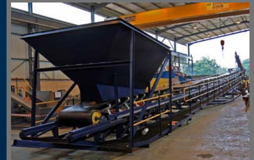
300 TPH Coal Conveyor
