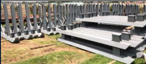
Overland Ash Dump Modular Conveyor System
