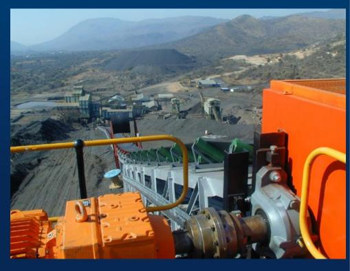
The design, manufacture and supply of a 1500m long x 1500mm wide Overland Conveyor.
