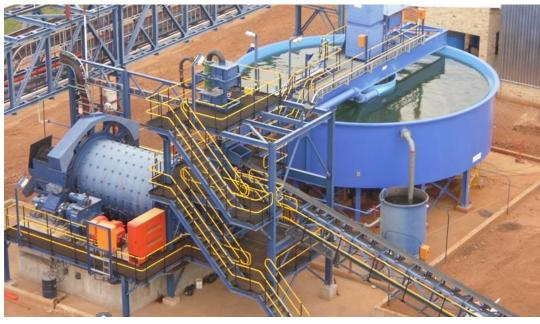
Ball Mill to Process Pyrolusite Turnkey Supply and Refurbishment, Installed and Commissioned
