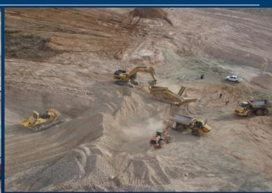
3 600 000 tpa Diamond Operation 6 x 40t ADT's, 6 x CAT 966 Front End Loaders, 1 x 475 Komatsu Dozer, 1 x D9 Cat Dozer, 1 x D10 Cat Dozer, 3 x Excavators (30-85t), 3 x Trommel – Spyder / Warrior Mobile In-Pit Screens, with mobile de-sanders 6 x Rotary Pan Plants 30 tph Dense Medium Separation Plant Modular X-Ray Recovery Plant
