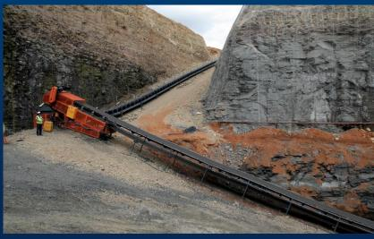
Pit to surface stockpile Project - Designed, Manufactured, Installed and Commissioned 1000 t/h Overland and Spreader Conveyor System, 600 t/h Garland Conveyor System
