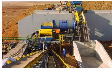
200t/h Dense Medium Separation Diamond Recovery Plant Scrubbing, DMS, XRay recovery Turnkey Supply, Installed and Commissioned
