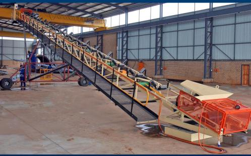
Multiple grass-hopper conveyors and one slewing/stacking conveyor for 25000 tons Uranium dumps Turnkey Supply Design Manufacture Logistics
