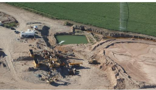
1,800,000 tpa Process Plant and Mining Operation Development Trommel Screens, De-sander Units, Mobile In-Pit Screens Rotary Pan Plants
