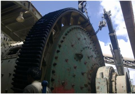
Design and manufacture of new girth gear and pinion Non destructive tests and heat treatment Installation
